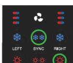
**To deactivate Split Fan Mode:** Use the remote control from either base to press and hold the Right Heating button and Sync Cooling button for 6 seconds. After 6 seconds, the remote backlight should blink 2X indicating the bases are no longer in Split Fan Mode. When Split Fan Mode is deactivated, the fan buttons on both remote controls will revert back to the default state where all fan buttons control all fans on sync'd bases.
